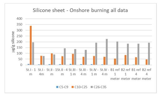
Figure 11. Fractions of the oil (C5-C9, C10-C25, C26-C35) as incorporated in silicone sheets beneath the in situ burning operation (St. I - St. IV, screw numbers in the horisontal transect at lowest tide level) and in the reference bay (ref). The lighter fraction is somewhat elevated in the in situ burning bay compared to those in the reference bay.
